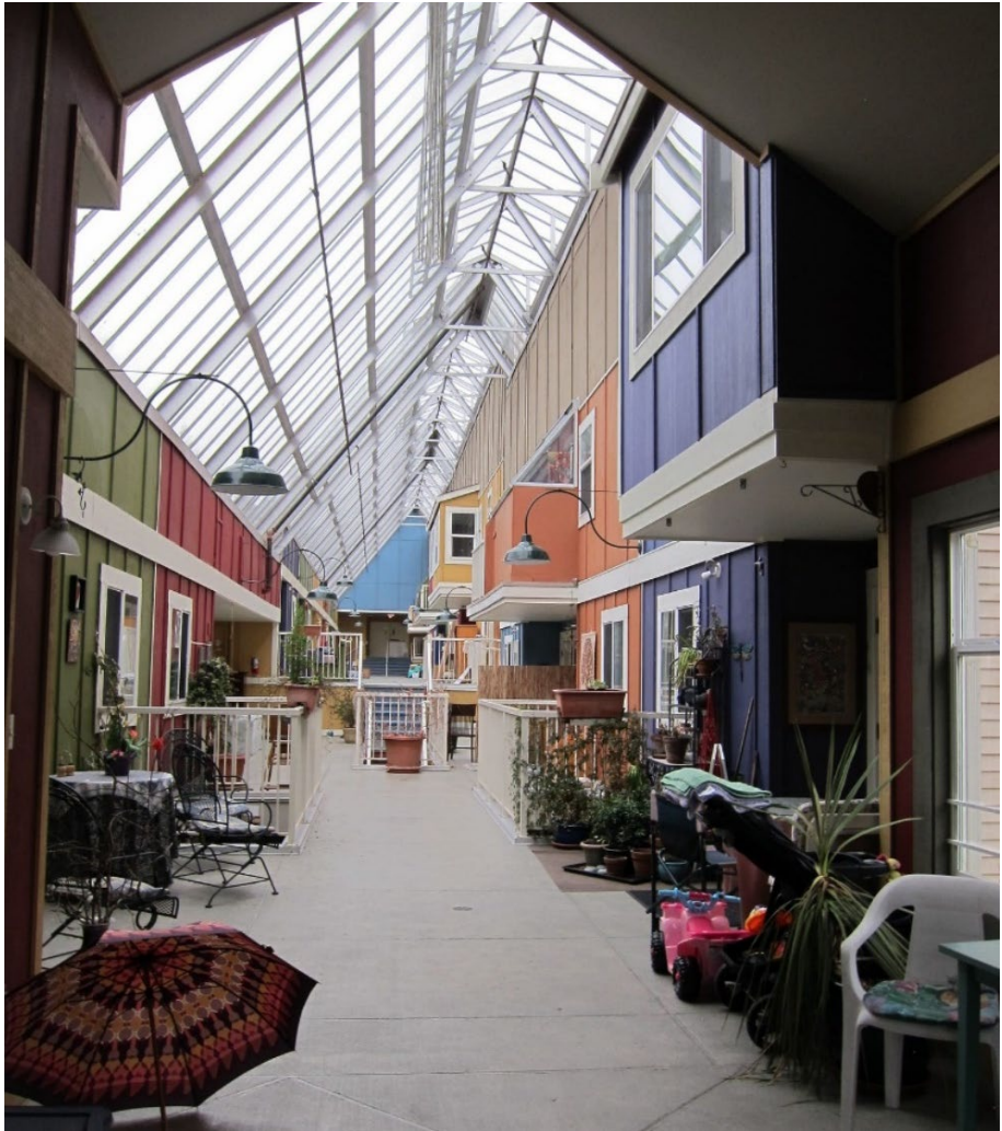
Figure 4.63 At WindSong Cohousing Community in Denmark an indoor-outdoor street makes the circulation space more comfortable year-round. This increases the use of transitions zones leading to more spontaneous interactions [9].
